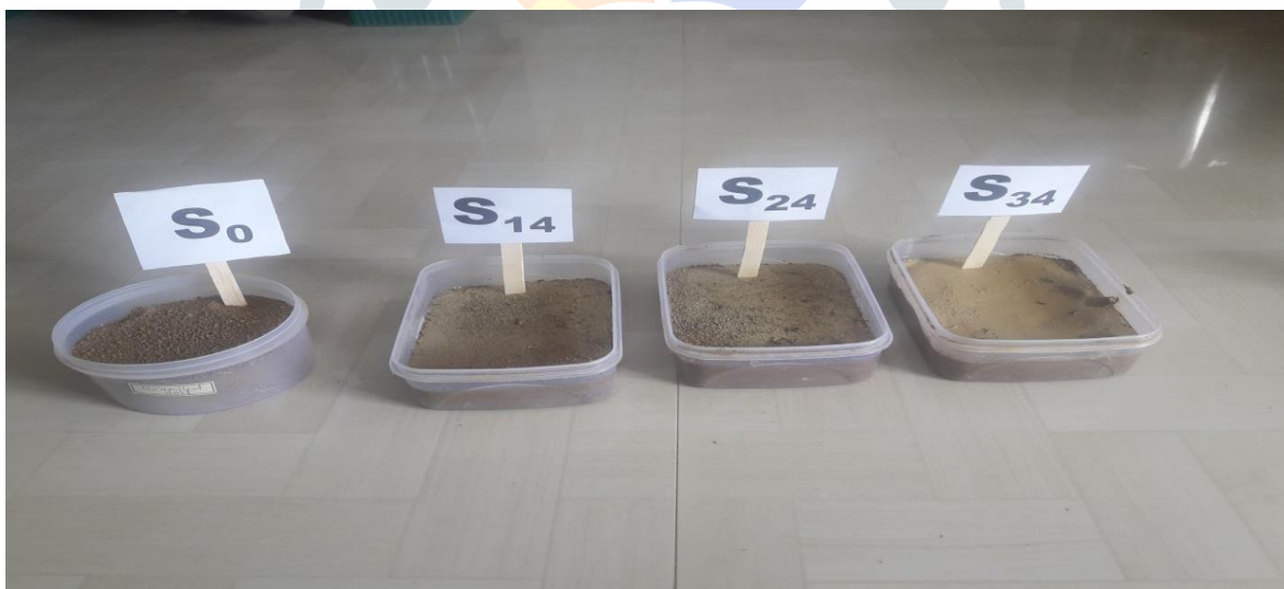
Fig 5 Photography of controlled soil, 4mM, 5mM and 7mM aqueous ALS with 0.03mM sodium hypochlorite
