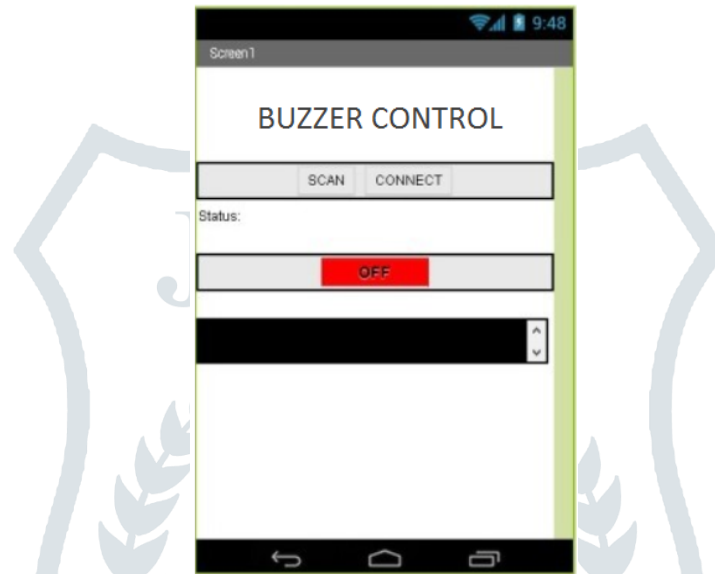
Figure-5.Mobile app for connect BLE and buzzer control indication.
