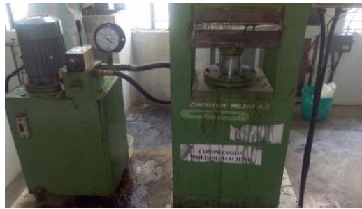
Figure 6. Curing in Compression Molding Machine
