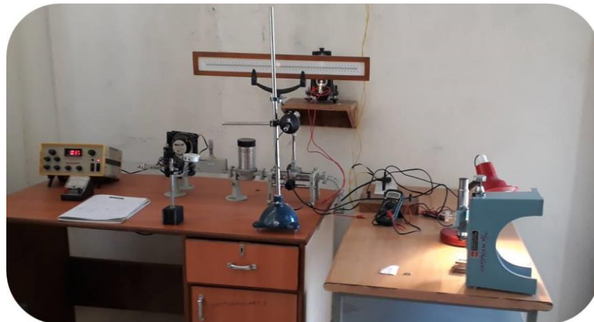
Figure:-1 X-Band Microwave bench set up
