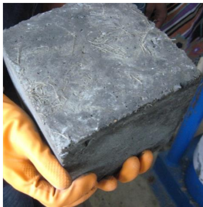
Fig.4.2.Casted concrete fiber cube
