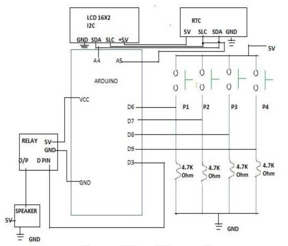
In the above circuit the power to the device is given by either solar panel or 230v power supply through adapter (Dc power supply 12-15v) and controlled by +5v given by reference clock. The push button is used to
