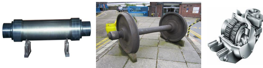
Fig 1.1 (a)Rail axle, (b)wheel set, (c)axle box
