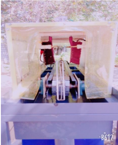
Fig -1: Internal view of dishwasher
