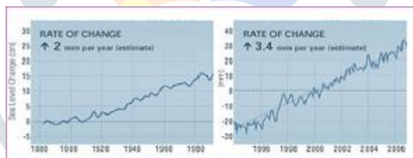
Figure 2. Mean annual sea level rise associated with the thermal expansion of sea water due to warming and widespread melting of ice sheets. Left chart: Historical sea level data derived from 23 tide-gauge measurements. Right chart: Average sea level since 1993 derived from global satellite measurements (NASA, 2009).
