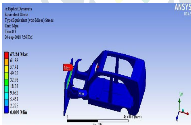
Figure 13 Von-Mises Stress of Al 6061 Frame with Spring Steel Honeycomb Structure Bumper
