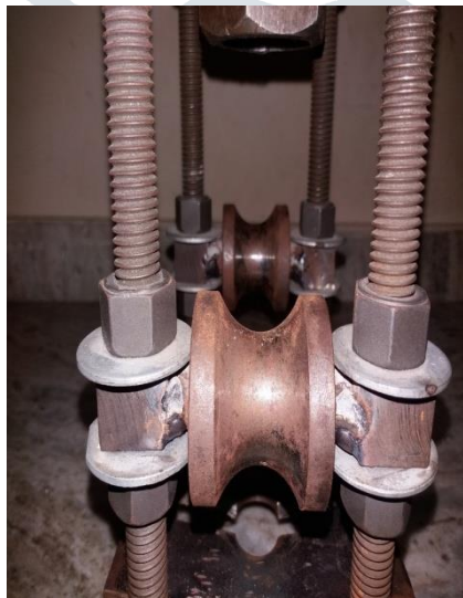
Fig. 4: Pipe bending arrangement
