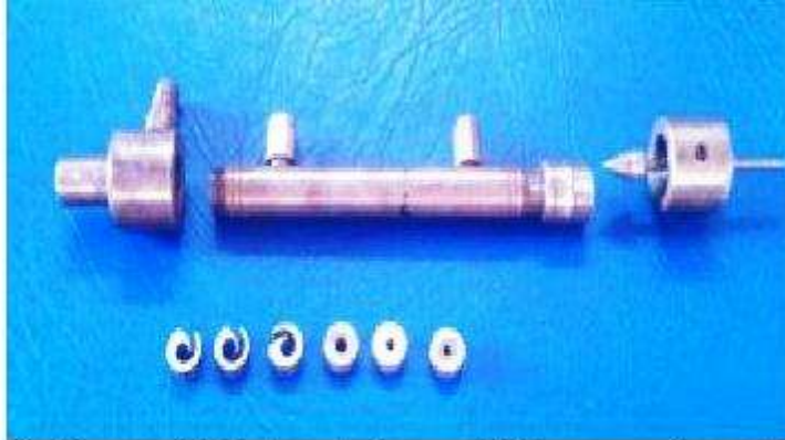
Fig 2: Parts of Vortex tube used for experimentation
