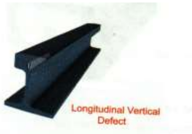
Fig. 2 - Schematic Diagram for Longitudinal Vertical Flaw
