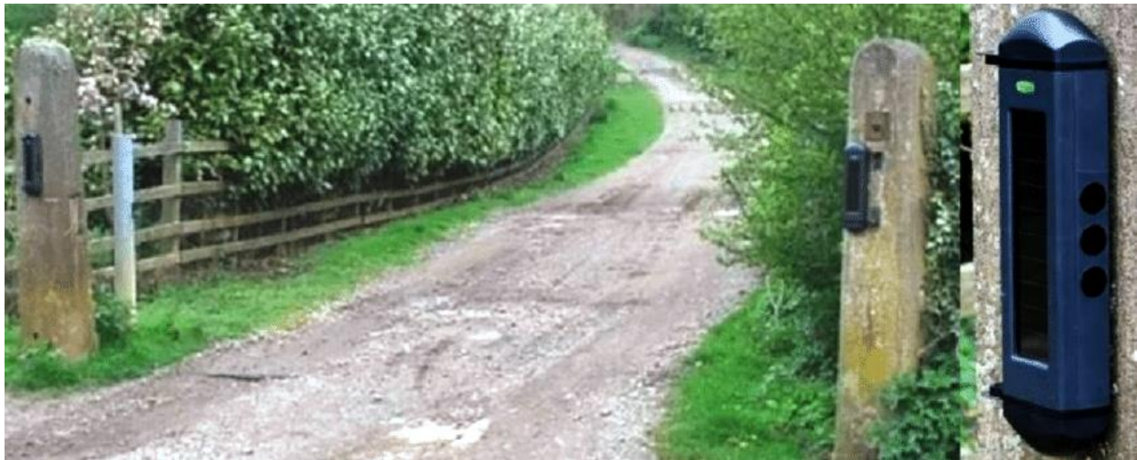
FIGURE 4: AN IR BARRIER WITH A COMPREHENSIVE VIEW OF AN OPTOELECTRONIC SENSOR / TRANSMITTER.
