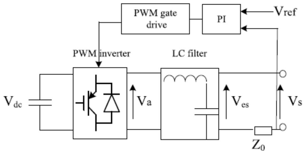
Fig. 5 ES with voltage control loop
