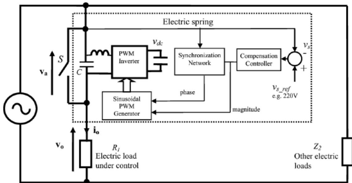
Fig 6 The experimental setup for the electric spring (with control block diagram)
