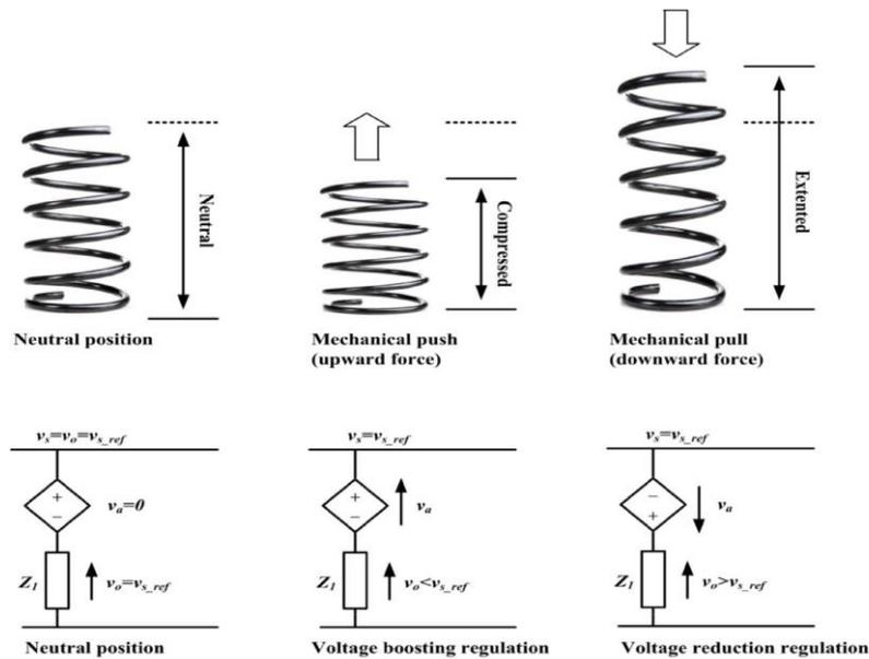
Fig.1. Analogy of a mechanical spring and an electric spring
