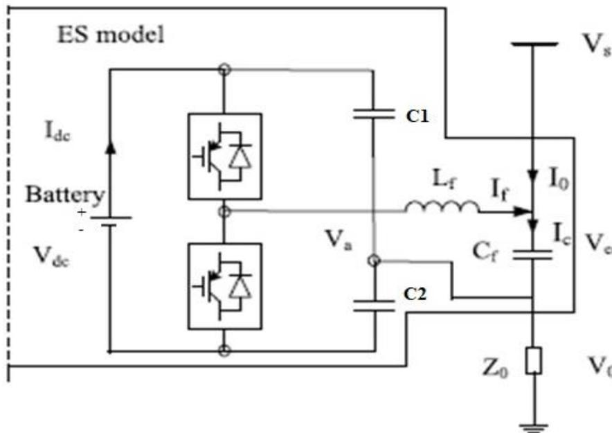
Fig.4. Circuit diagram of the ES
