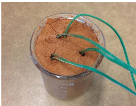
Figure 4. Watermark sensors in soil container.
