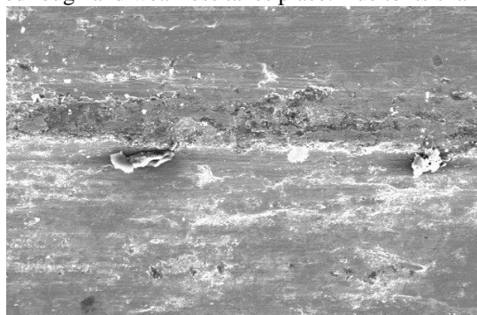
Fig 6.3. SEM micro graph of Sp-4, Speed-2.45m/s, applied load 20 N.
