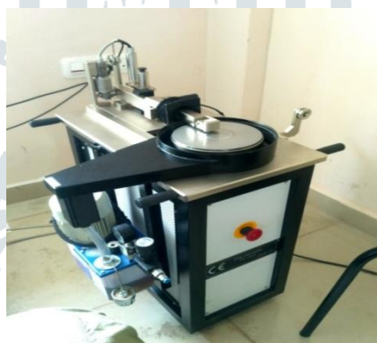
Fig. 5.4 Ducom pin on Disc sliding wear test apparatus
