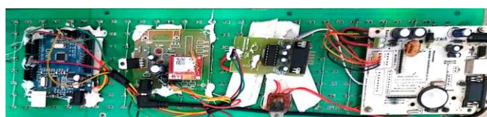
Figure4: Arduino Board interfacing with GSM and LED Display
