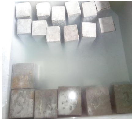
Fig 8: Specimens in curing tank
