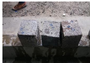
Figure: 11 Acid cured cube
