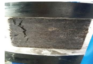
Figure: 12 Strength test of Acid cured cube
