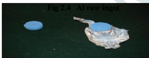
Fig 2.4 Al raw ingot Fig 2.6: Degasser hexachloroethane \text{C}_2\text{Cl}_6 tablet
