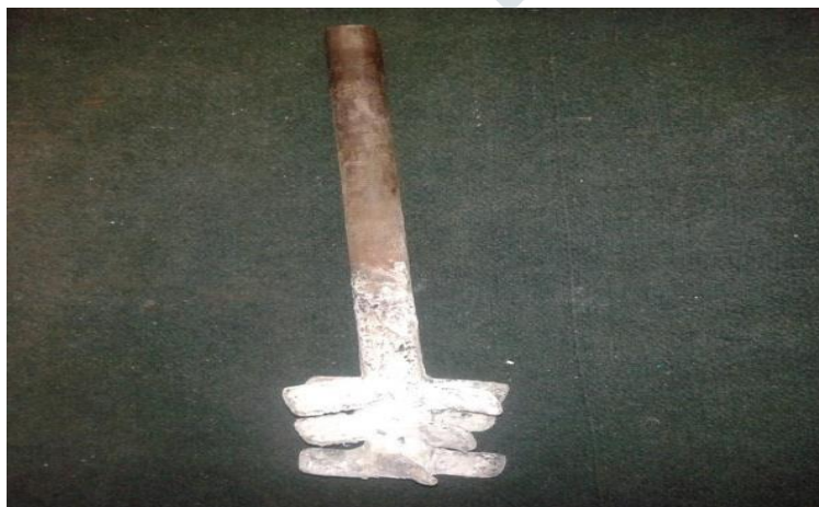
Fig 2.3: Alumina- sodium silicate powder coated stirrer
