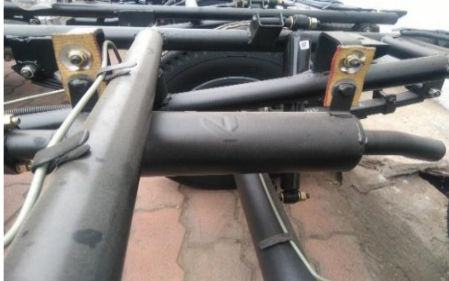
Fig 2: Figure exhaust system engine assembly
