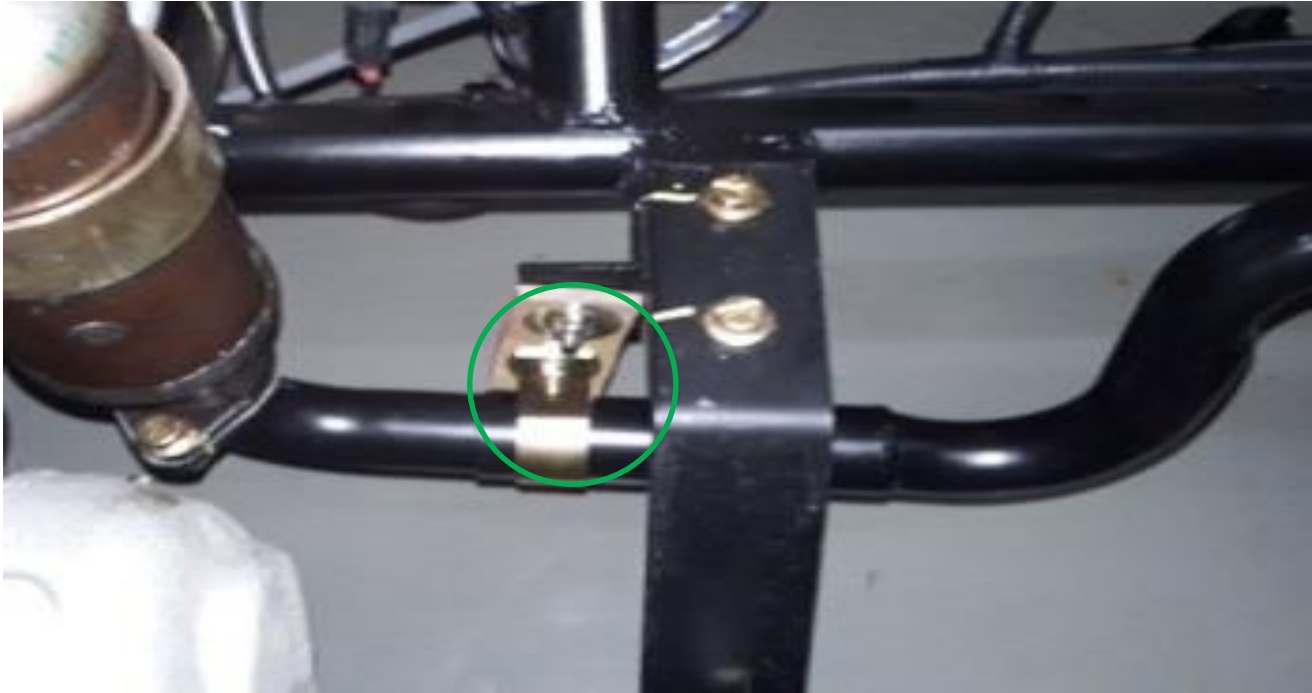
Fig 8: Figure Exhaust mounting before
