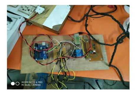
In this project we are using a Arduino UNO, 3 relay(1st for motor,2nd for solenoid valve and 3rd for future use),One solenoid valve,one motor, five float sensors and a power supply of 12v DC for solenoid valve.
