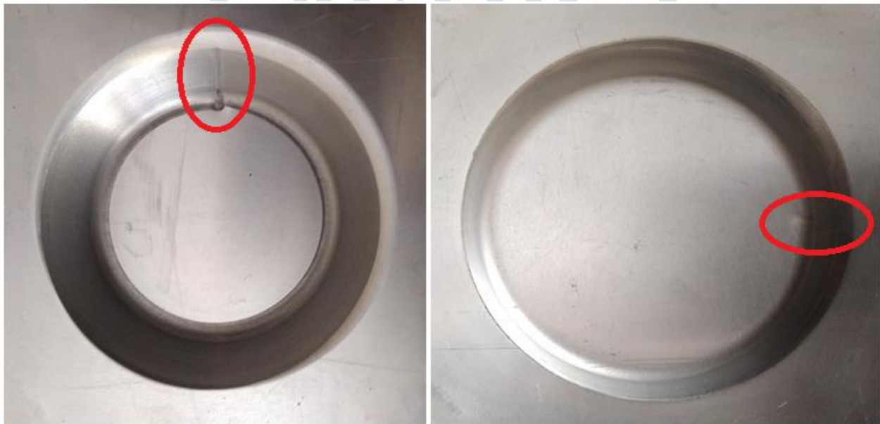
Figure No. 10 Truncated Cone manufactured from Contour tool path [Height 20mm, Wall angle 60^\circ , Dia 100 mm]
