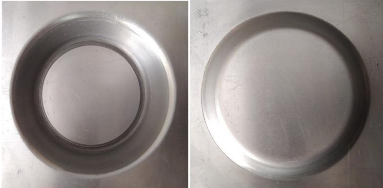
Figure No. 9 Truncated Cone manufactured from Spiral tool path [Height 20mm, Wall angle 60^\circ , Dia 100 mm]
