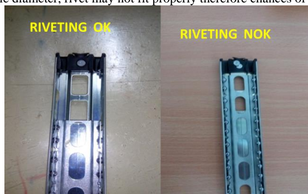
Figure 2.12 Riveting of End Stopper (Ok & Not Ok parts).
