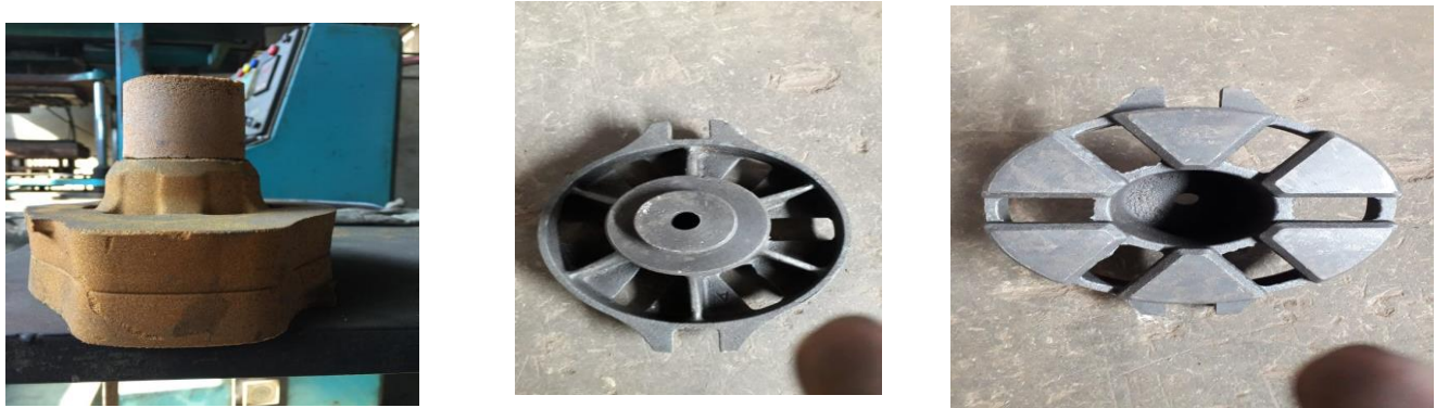
Figure 4 85mm runner height and 34mm runner weight
