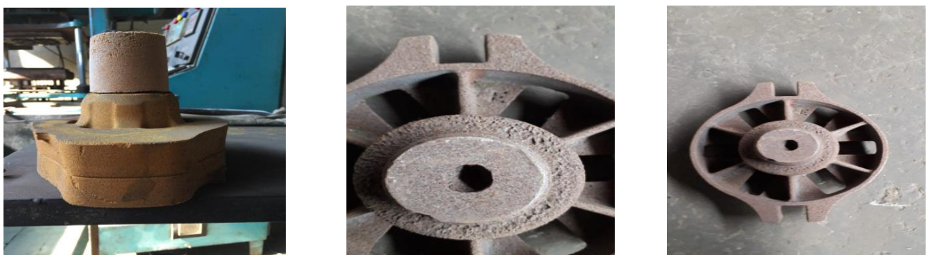
Figure 3 90mm runner height and 37mm runner weight
