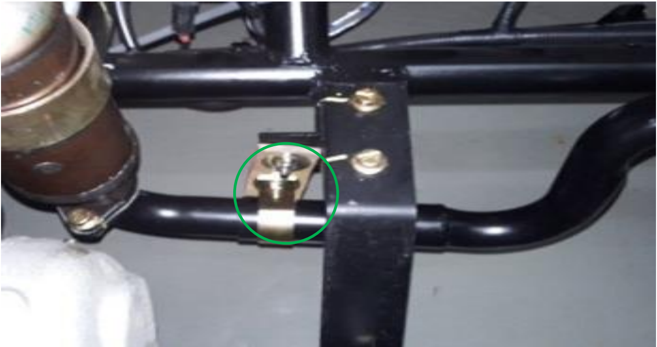
Fig 8: Figure Exhaust mounting before
