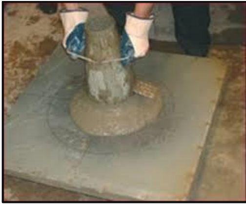
Fig 2 :- Slump Flow Test
