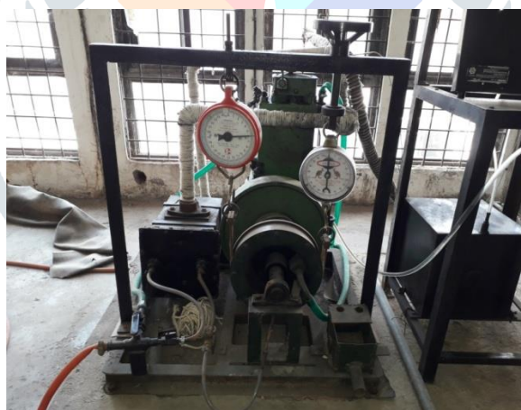
Fig. 1 Engine set up [1]
