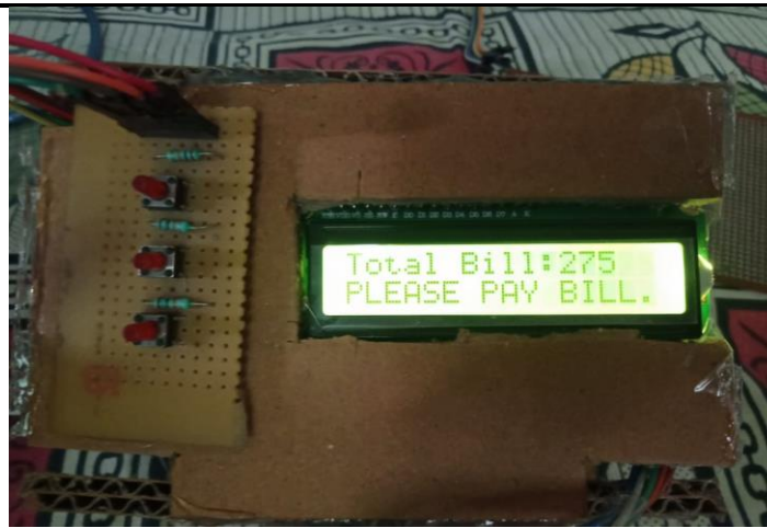
Figure 11 When middle button is pushed Total bill is displayed
