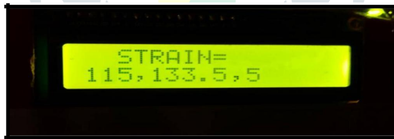
Fig. 11: Strain gauge value for hub drum
