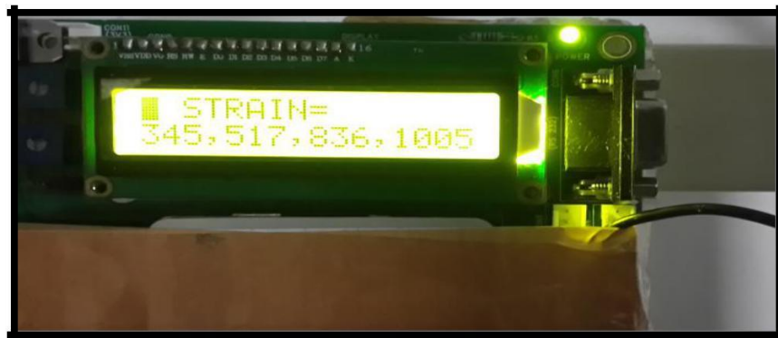
Fig. 13: Strain gauge value for gusset
