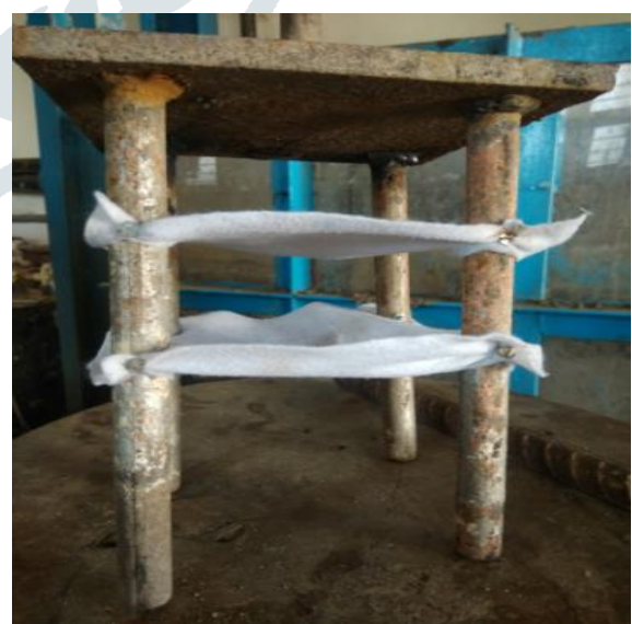
Fig 6 Four piles with double geotextile layer
