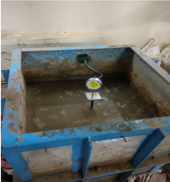
Fig 3 Set up for the heaving test with dial gauge Arrangement
