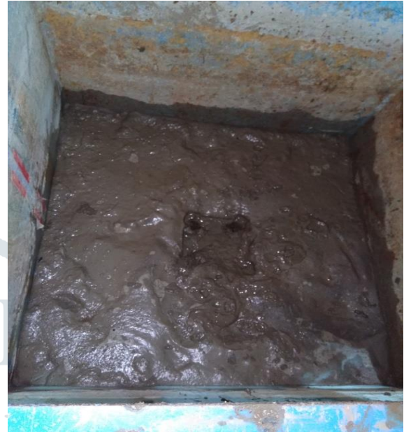
Fig 4 Heaving of soil after 4 days
