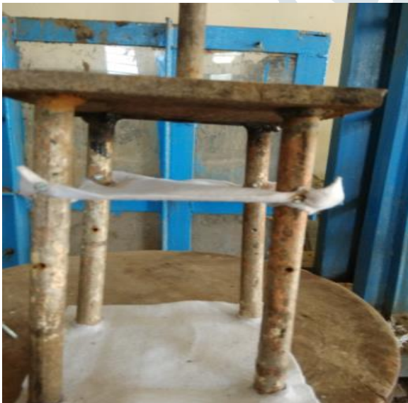
Fig 5 Four piles with single geotextile layer
