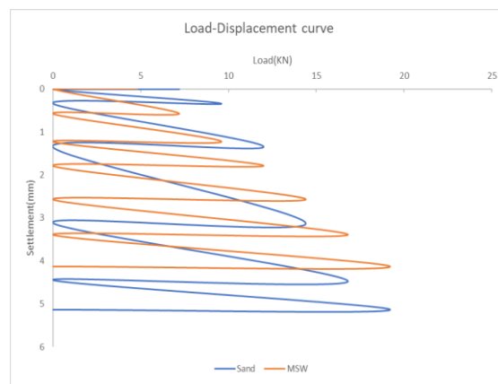
Fig. 5: Load v/s Displacement characteristics for Sand and MSW at dialgauge location H3
