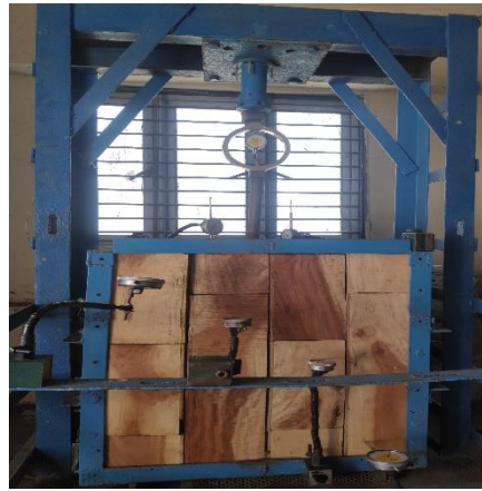
Fig. 2: Reinforced wall test setup
