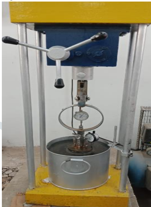
Fig 3: Setup for measuring swelling pressure in the constant volume method
