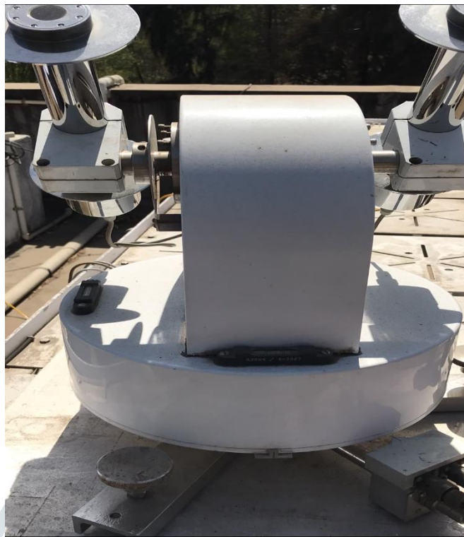
Fig 2.Pyrheliometer mounted on a solar tracker.
