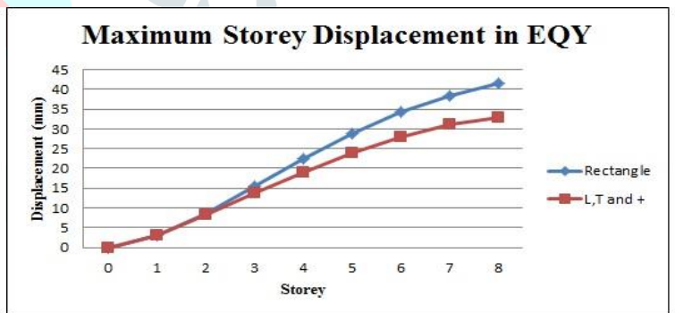
Figure 4: Maximum Storey Displacement in EQY in G+7 storey building
