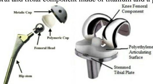
Fig.1 schematic diagram of artificial hip joint (left) and knee implant (right) [53]
