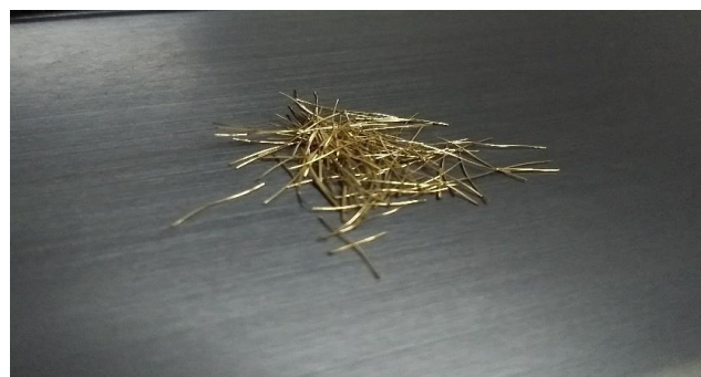
Figure 1: Brass Coated Micro Steel Fibre (13 mm)
