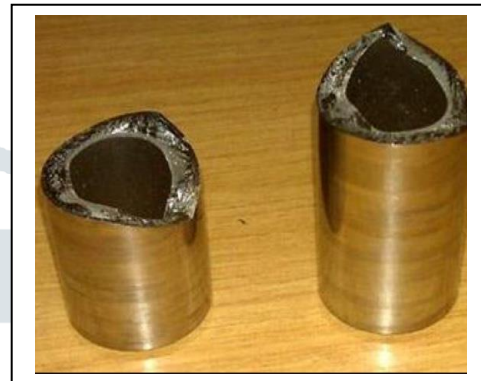
Fig 3 Damaged piston pin [2]
