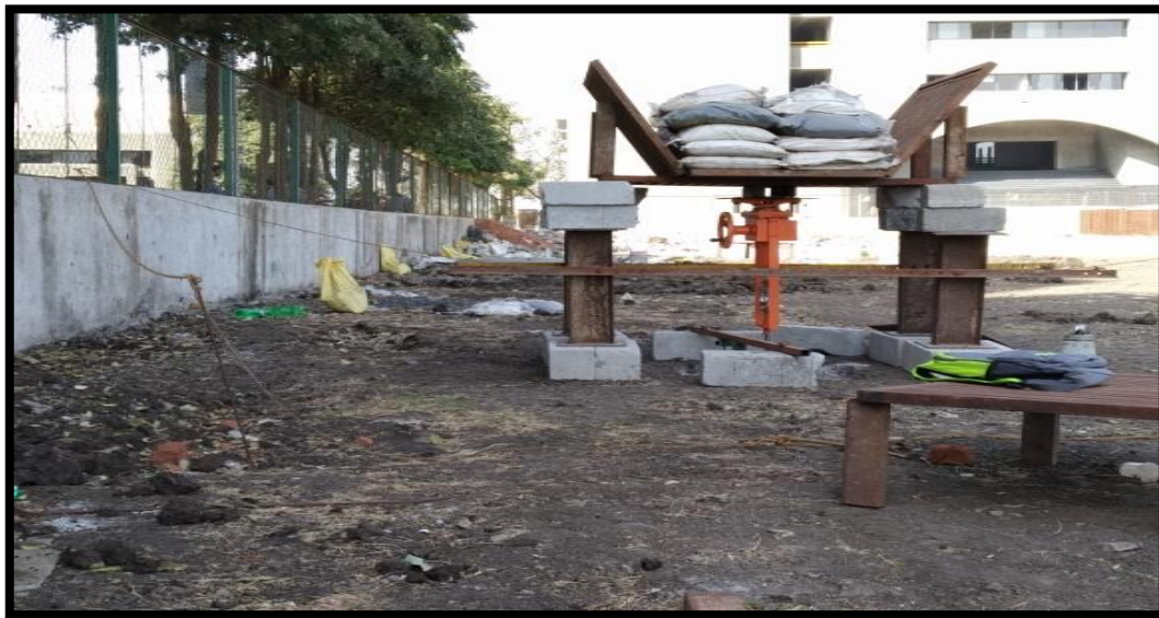
Fig 2. Field C.B.R setup
