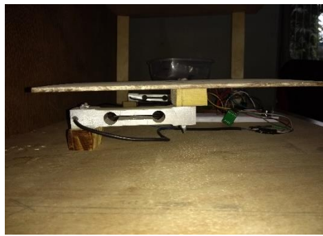
Fig.3 plate fixed on load cell
