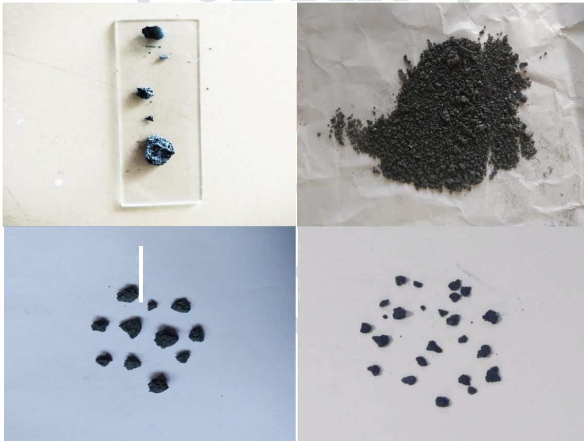
Fig. 2 grown crystals using zone levelling method
