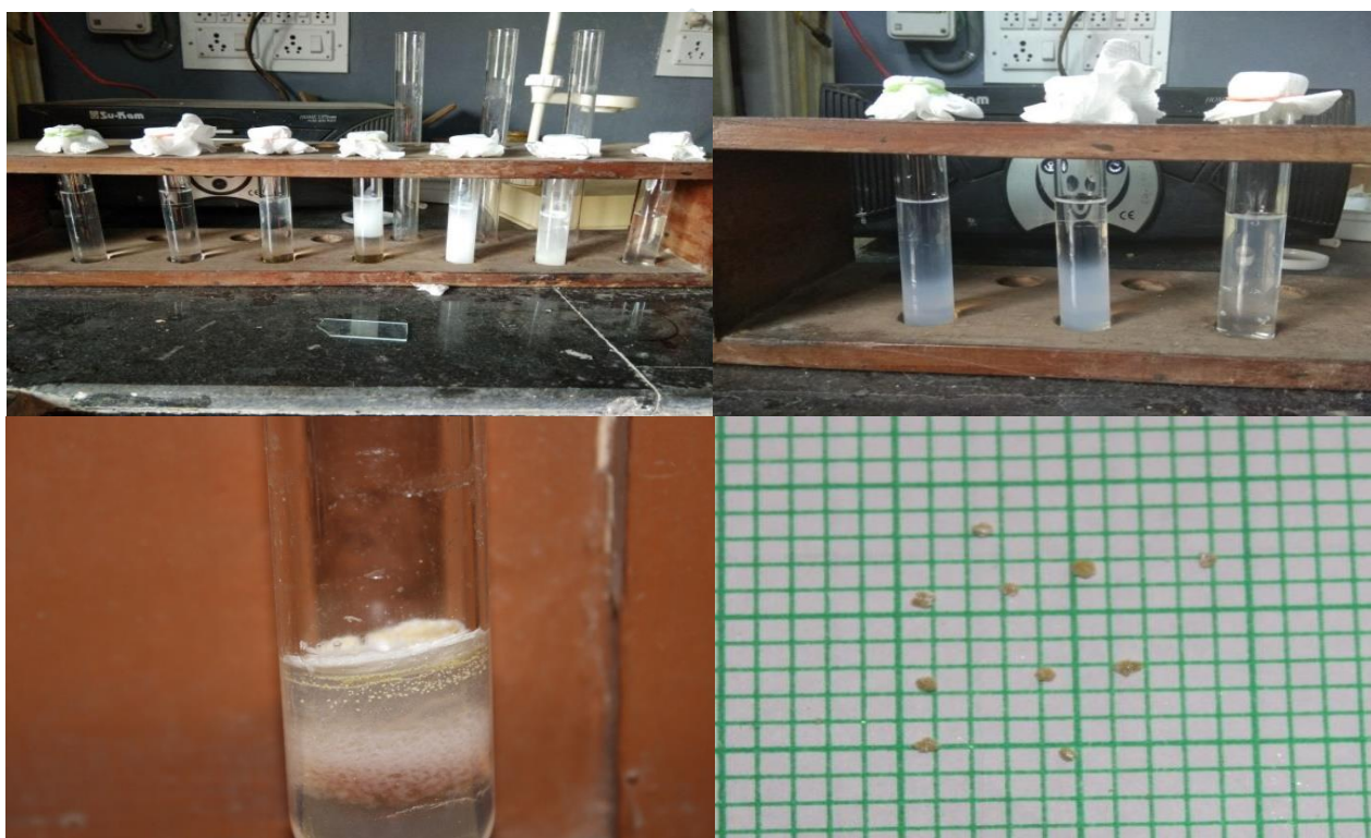
fig.3 gel method and gel grown crystals
