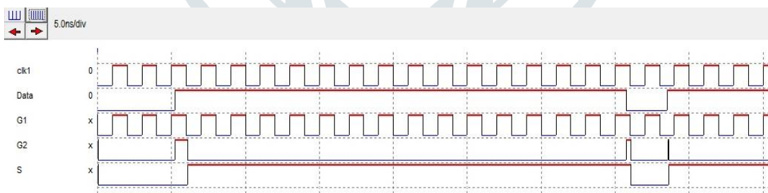
Fig. 16: Simulation of D-Flip Flop Using MSH Gate
