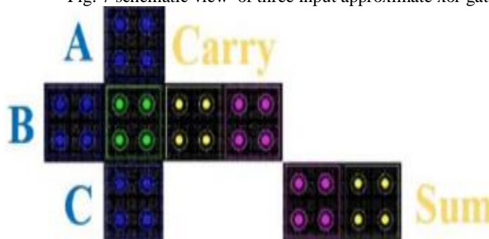
Fig. 7 schematic view of three input approximate xor gate
