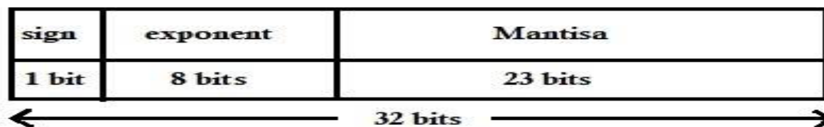
Figure1. IEEE 754 single precision format
