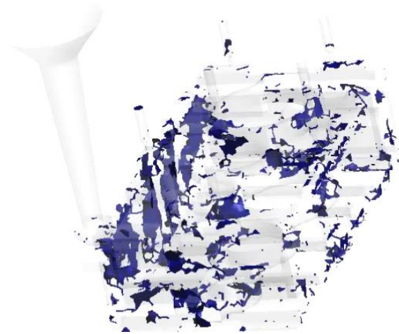
Fig. 7.10 Cold shuts defect accruing in part
