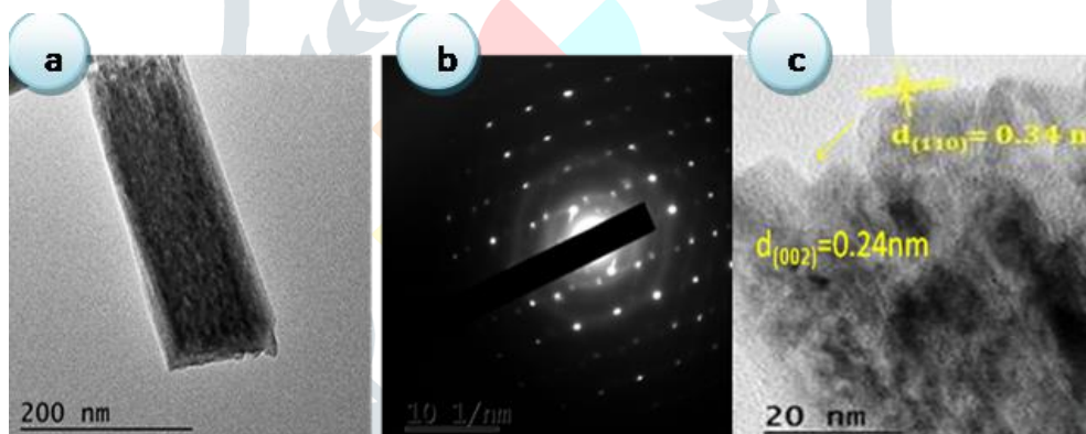
Fig.3 (a) shows TEM image, (b) SAED pattern and (c) HRTEM image of TiO 2 - ZnO sample.
