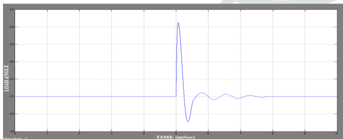
Fig.11 Generator load angle D_{YX} , during fault and after fault by using single line scheme
