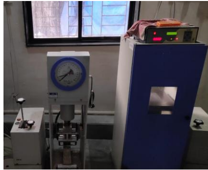
Fig. 2.2.5. Flexural and split tensile strength test apparatus
