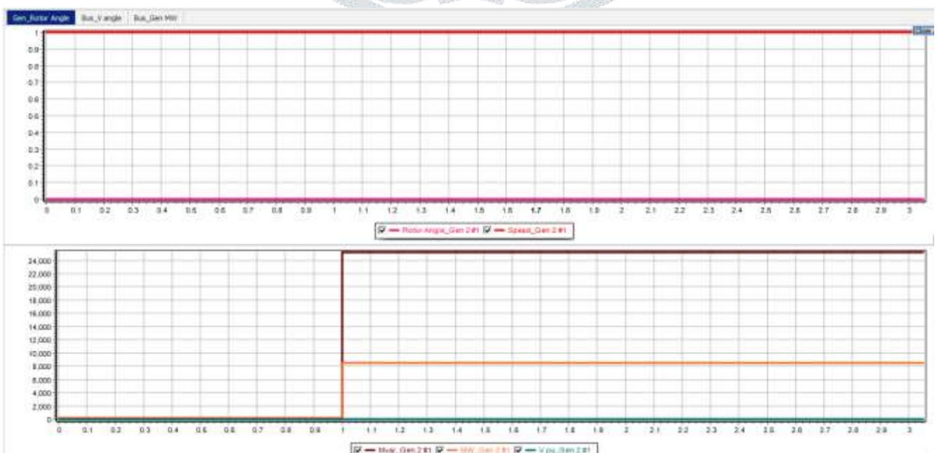
Figure 5 Gives Speed of the generator during Mismatch, Rotor Angle Swing, MVAR rise, MW step change during Fault Occurrence
